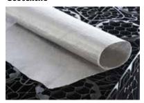
Permeable geotextiles are for use in infiltration applications. They permit the passage of water into and out of the ACO StormBrixx® system. Geotextiles are also used to protect the geomembrane from mechanical damage due to ground and thermal movement. They are placed on the outer side of geomembrane.
